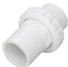
*The Plumbing Unions connect the plumbing lines to the components. Unions can become loose in transit and when seasons change. During the initial installation and each time you drain your spa, you should hand tighten all plumbing unions. The main cause of leaks inside the spa cabinet is plumbing unions that need to be tightened or seals that need to be re seated or replaced. Do not use tools or overtighten plumbing unions.*
